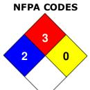
NFPA 30 / 30B Storage Classification: Flammable Liquid IB
